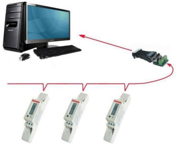
Configure IndigoSCADA with a new modbus RTU unit with the following modbus database: Taking the register address minus 30001 : so for Total Kwh. 30343 minus 30001 = offset address is 342
