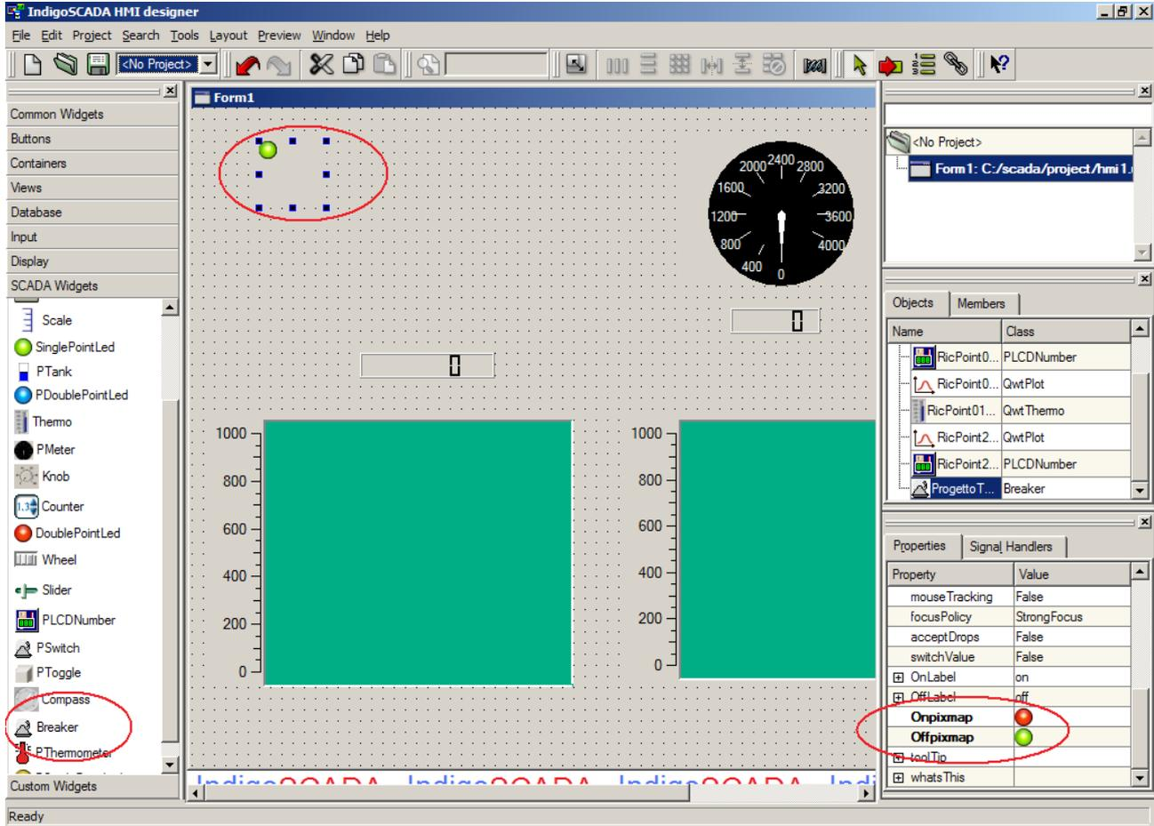
Use **DoubleBreaker** widget to animate double points bitmaps. The bitmaps are selected in Properties Onpixmap, Offpixmap, Invalid11pixmap and Invalid00pixmap. Onpixmap is shown in HMI when the value of the point is 2. Offpixmap is shown in HMI when the value of the point is 1. Invalid11pixmap is shown in HMI when the value of the point is 3. Invalid00pixmap is shown in HMI when the value of the point is 0.
