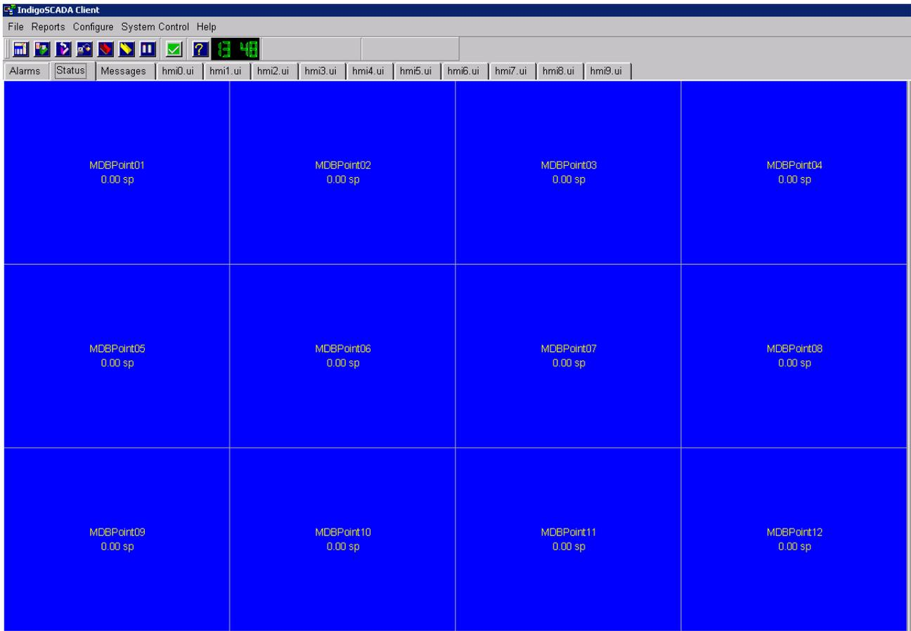
We used 24 items of data in the Unit options **MDB** because **IndigoSCADA** comes already with a predefined set of 24 Modbus points, (named **MDBPoint01**, **MDBPoint02**, etc.) for quickly test it with **PeakHMI**.
