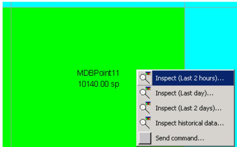
**IndigoSCADA Client** allows to inspect data in order to analyze the data and observe the trend of the process data. Go to the **Status** tab and right-click inside one the rectangles representing process data (e.g **MDBPoint11**) and choose **Inspect last two hours** for example.
