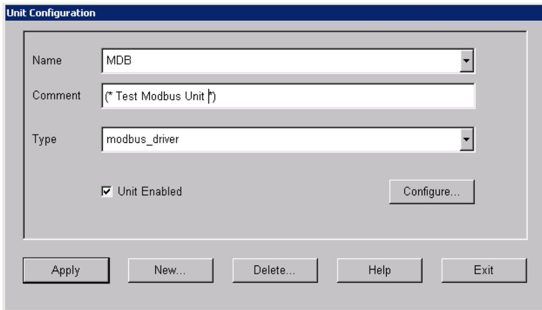
Choose **modbus\_driver** as Type and press the **Configure** button to set some specific options. Select **TCP** as Context, **127.0.0.1** as IP address, **502** as Port, **24** is the number of total sampling points (N items) belonging to this unit and **1000** ms as Poll interval.
