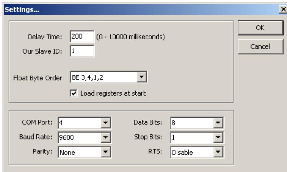
In IndigoSCADA select **RTU** as Context, **COM3** as Serial device, **9600** as Baud, **8** as Data bits, **1** as stop bit, **N** as parity (N= None, E= Even, O= Odd parity), **24** is the number of total sampling points (N items) belonging to this unit and **1000** ms as Poll interval.
