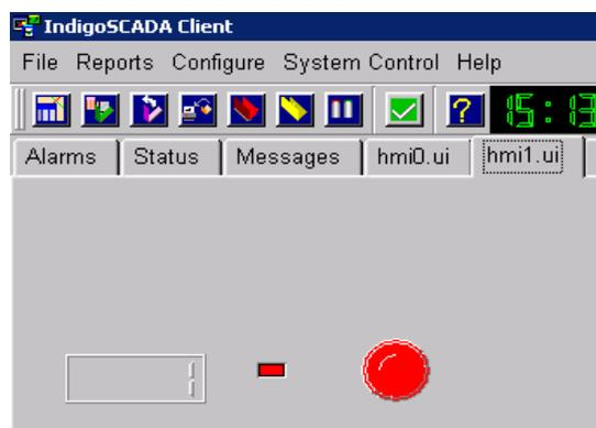
The graphic object will begin to flash because Point is in alarm state. Press the **Acknowledge All Alarms** button to stop the animation.
