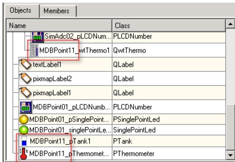
Set type of MDBPoint11 to `M_ME_TE_1`, accordingly to **modbus\_database1.db** column `iec_type_read`.
