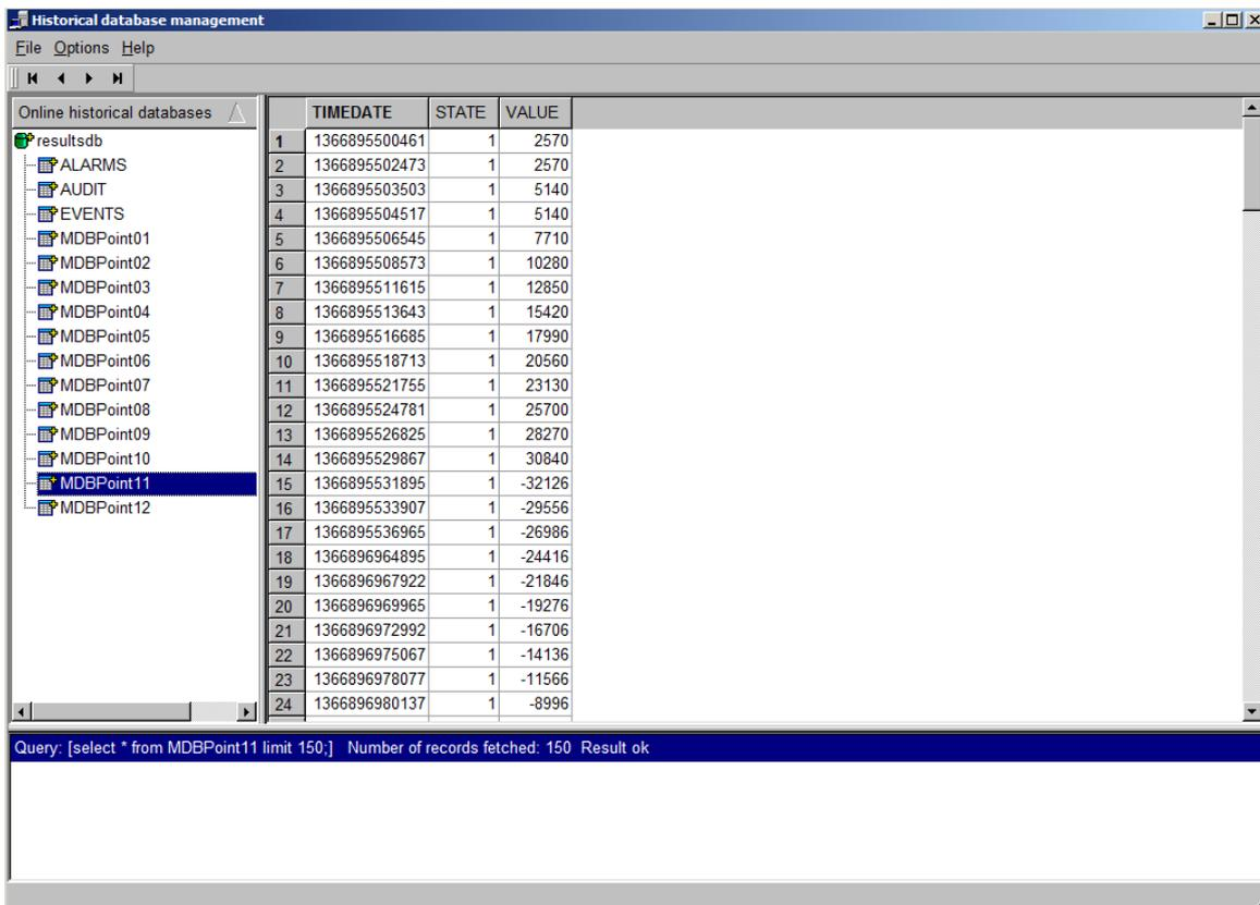
Historical database management is used to analyze all the process data samples from the beginning. It gives a low level access to all internal tables of **IndigoSCADA**
