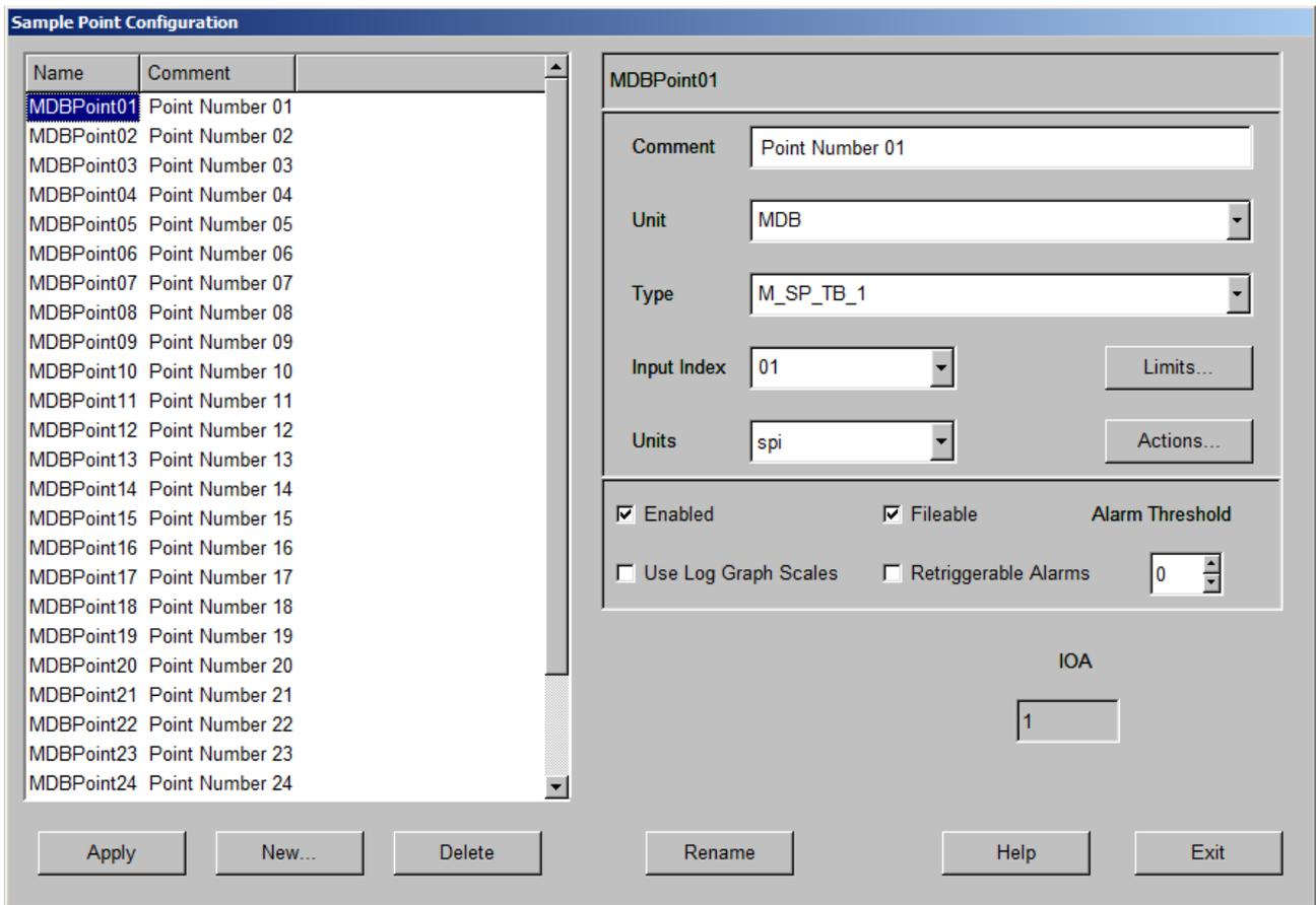
press "Limits..." button and set the value of the single point (0 or 1) to associate with the alarm state. In the next picture the value of 1 gives an alarm state.
