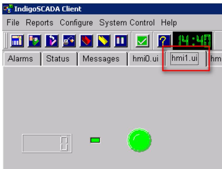
Save the map and exit **IndigoSCADA Client** by choosing **Exit** from the **File** menu, After few seconds, the client will be opened again and in the **hmi1.ui** tab those three new objects will be inside.
