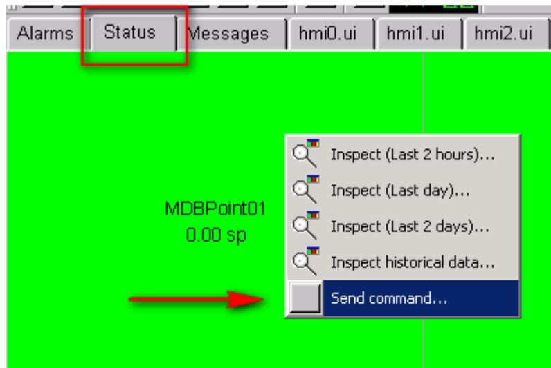
Write 1 in the **Value** text box and press **OK** button. The rectangle will become light blue and in the right part of the window a new Alarm will be notified.
